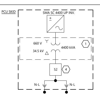
1. STEP-UP TRANSFORMERS ARE OWNER FURNISHED AND INSTALLED BY MANUFACTURER WITHIN PCU STATION. PCU STATION DESIGNED AND ASSEMBLED BY OTHERS AND SHOWN FOR REFERENCE ONLY. TRANSFORMER PRIMARY PROVIDED WITH 600A NON-LOAD (N-L) BREAK TERMINATIONS. CONTRACTOR TO PROVIDE LOAD-BREAK (L) REDUCING TAP BUSHINGS FOR LOAD-BREAK ELBOW CONNECTIONS
