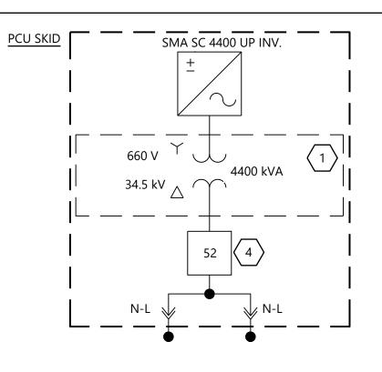
1. STEP-UP TRANSFORMERS ARE OWNER FURNISHED AND INSTALLED BY MANUFACTURER WITHIN PCU STATION. PCU STATION DESIGNED AND ASSEMBLED BY OTHERS AND SHOWN FOR REFERENCE ONLY. 2. TRANSFORMER PRIMARY PROVIDED WITH 600A NON-LOAD (N-L) BREAK TERMINATIONS. CONTRACTOR TO PROVIDE LOAD-BREAK (L) REDUCING TAP BUSHINGS FOR LOAD-BREAK ELBOW CONNECTIONS
