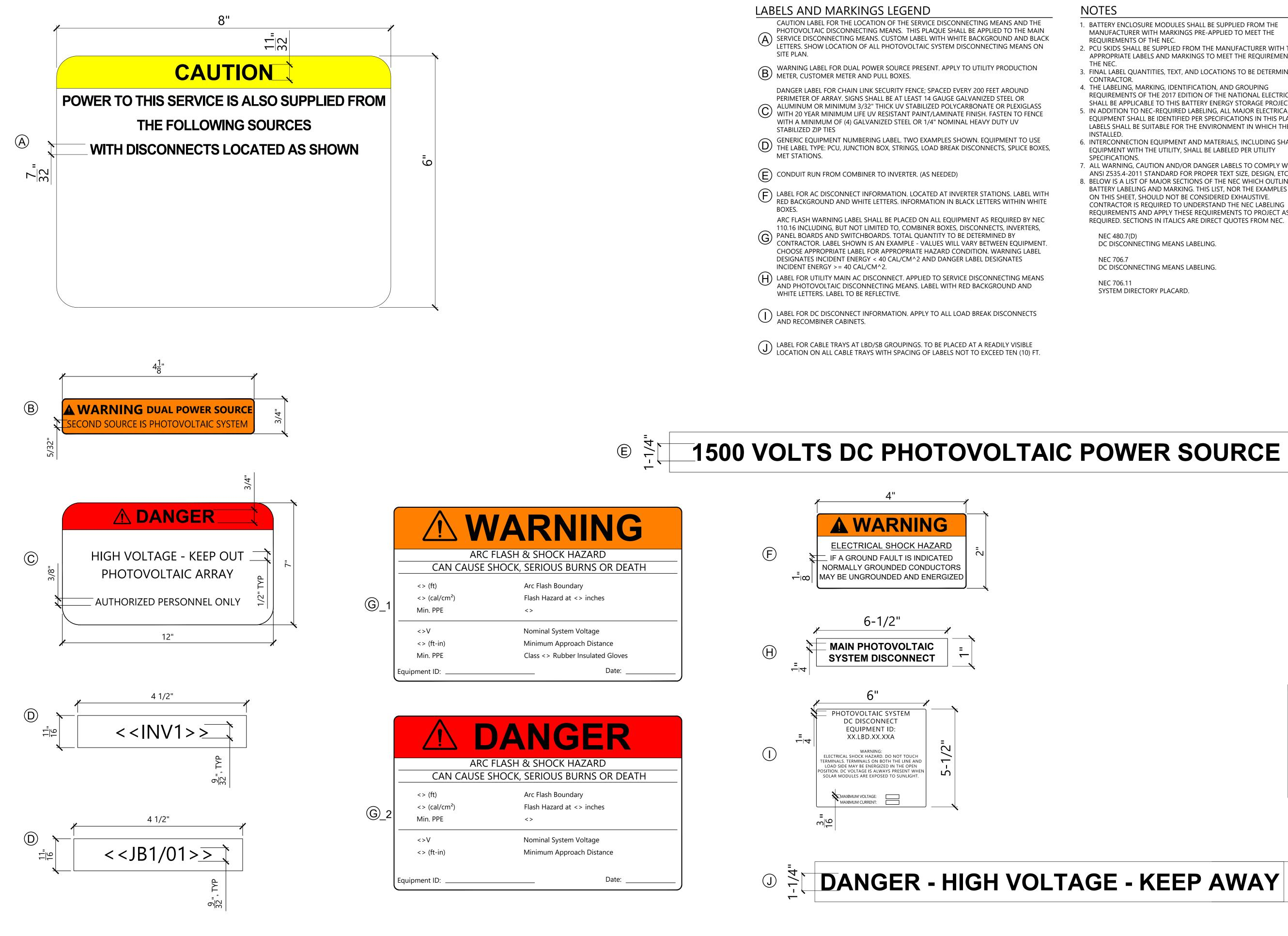
**1500 VOLTS DC PHOTOVOLTAIC POWER SOURCE**
