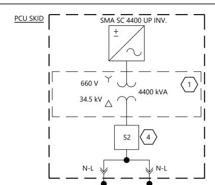
1. STEP-UP TRANSFORMERS ARE OWNER FURNISHED AND INSTALLED BY MANUFACTURER WITHIN PCU STATION. PCU STATION DESIGNED AND ASSEMBLED BY OTHERS AND SHOWN FOR REFERENCE ONLY. 2. TRANSFORMER PRIMARY PROVIDED WITH 600A NON-LOAD (N-L) BREAK TERMINATIONS. CONTRACTOR TO PROVIDE LOAD-BREAK (L) REDUCING TAP BUSHINGS FOR LOAD-BREAK ELBOW CONNECTIONS
